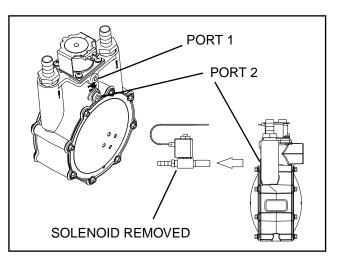
Figure 19 (10 kW) Gas Pressure Test point
